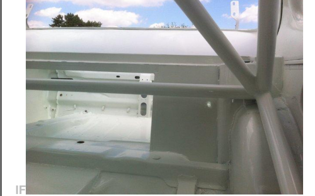
PHOTO 13 SHOULDER HARNESS ATTACHMENT – DRIVER
