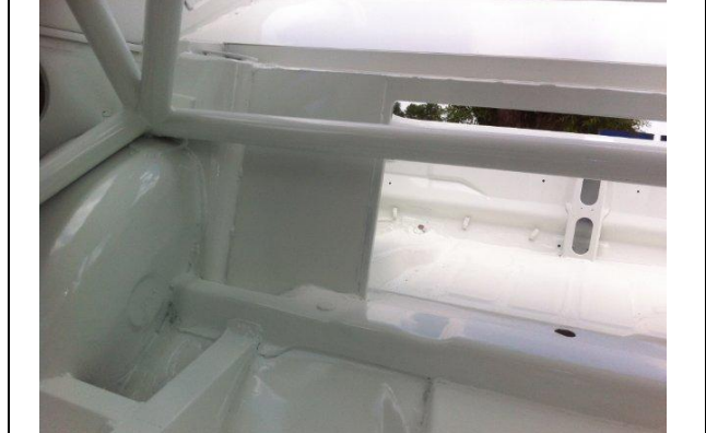
PHOTO 14 SHOULDER HARNESS ATTACHMENT – CO-DRIVER
